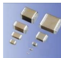
Ultra-small, high-capacity ceramic capacitors
