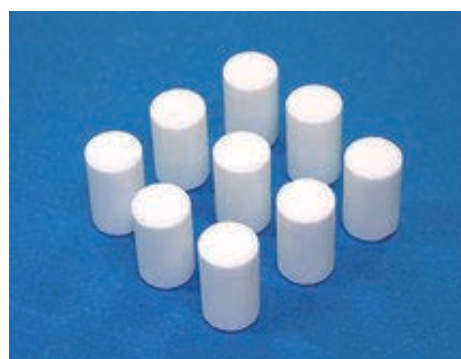
Clear encapsulation material for LED devices
